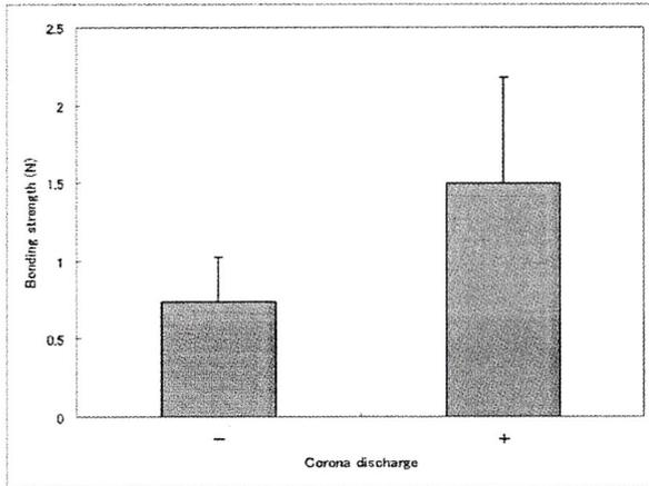
Figure 3. Bonding strength between the gelatin hydrogel coated and the surface of MM with (+) or without corona discharge (-).
