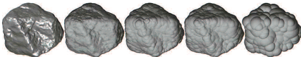
Figure 3.5 Simulation of real particle shape with overlapping spheres (after Ferrellec and McDowell 2010)
