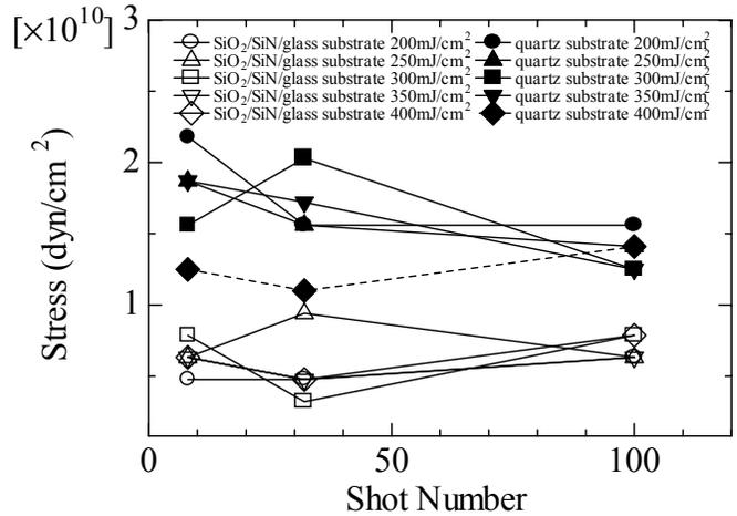
Fig.7 Relationship between the stress of the poly-Si and the shot number
