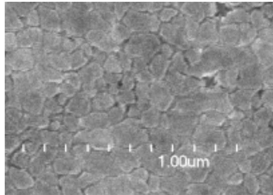
Fig.4 SEM photograph of poly-Si surface for the condition of  $400\text{mJ}/\text{cm}^2$  and 100 shots
