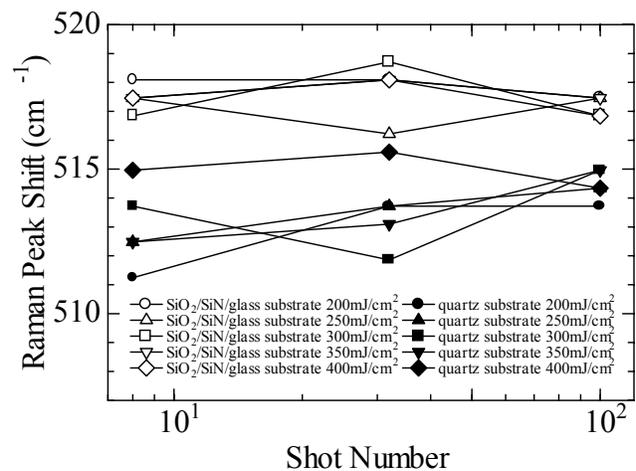
Fig.2 Relationship between the Raman peak shift and the shot number
