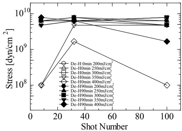
Fig.8 Relationship between the stress of poly-Si on the SiN substrate and the shot number
