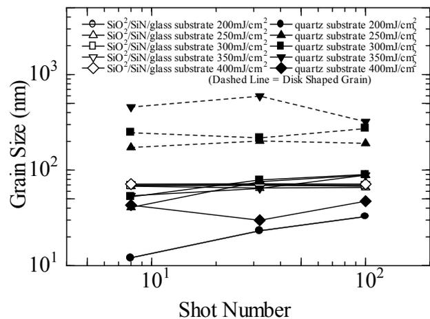
Fig.5 Relationship between the grain size and the shot number
