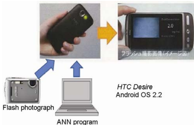
Figure 1. Dust measuring system using mobile phone camera.
