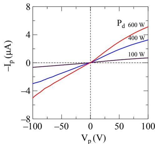
**FIGURE 3.** Typical  $I_p$ - $V_p$  characteristics in an ionic plasma in  $z > 0$  cm.
