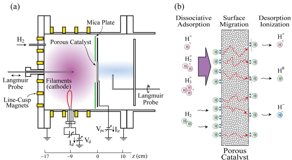
**FIGURE 1.** (a) Diagram of experimental setup for producing hydrogen pair ions on the basis of catalytic ionization. (b) Process of catalytic ionization under the positive-ion irradiation, which comprises dissociative adsorption, surface migration of hydrogen atoms, and desorption ionization.
