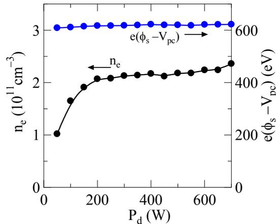
**FIGURE 2.** Dependence of the electron density and the irradiation energy of positive ions on the discharge power in the discharge region.
