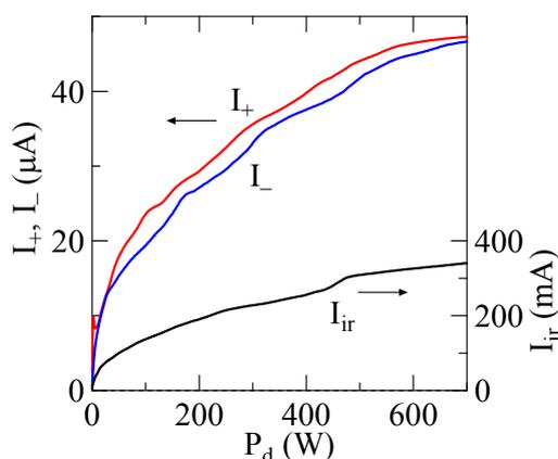
**FIGURE 4.** Production properties of  $H^+$  and  $H^-$  ions and irradiation current of positive ions as function of the discharge power.
