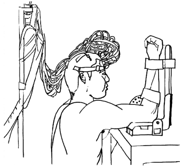
Figure 1 Experimental setup. Elbow flexion torque was measured in seated position. Both elbow and shoulder joint angle were set at 90 degree.
