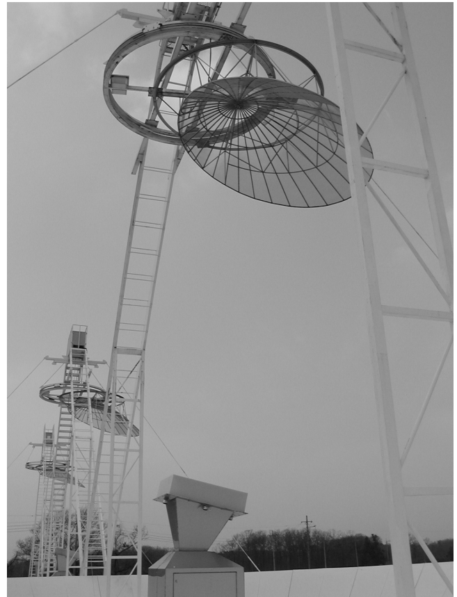
Fig. 3. Photograph of a sub-reflector and horn antenna equipped with a 20-m spherical antenna. Both rotate synchronously around the vertex axis of the sphere. The elevation angle is fixed at 85^\circ .
