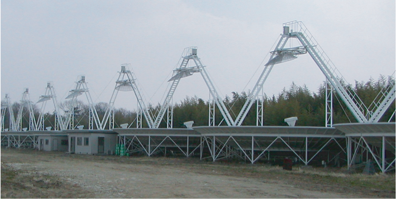
Fig. 2. Photograph of the array at Nasu Radio Interferometer. Eight equally spaced, 20-m diameter, fixed spherical antennas are shown in this figure.
