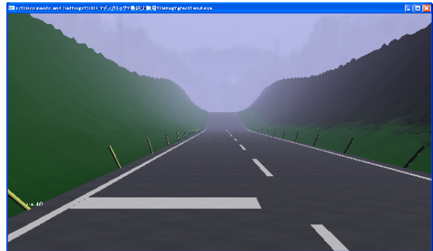
Figure 21. 1.4m tilt pole pattern of pole installation
