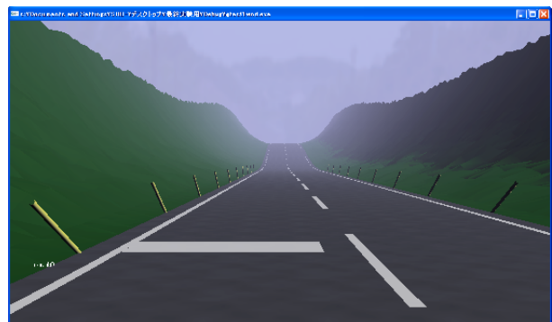
Figure 22. 1.7m tilt pole pattern of pole installation
