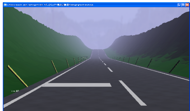
Figure 23. 2.0m tilt pole pattern of pole installation
