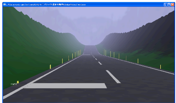
Figure8. inc.-P pattern of pole installation
