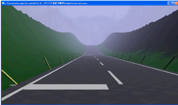
Figure11. tilt-P pattern of pole installation
