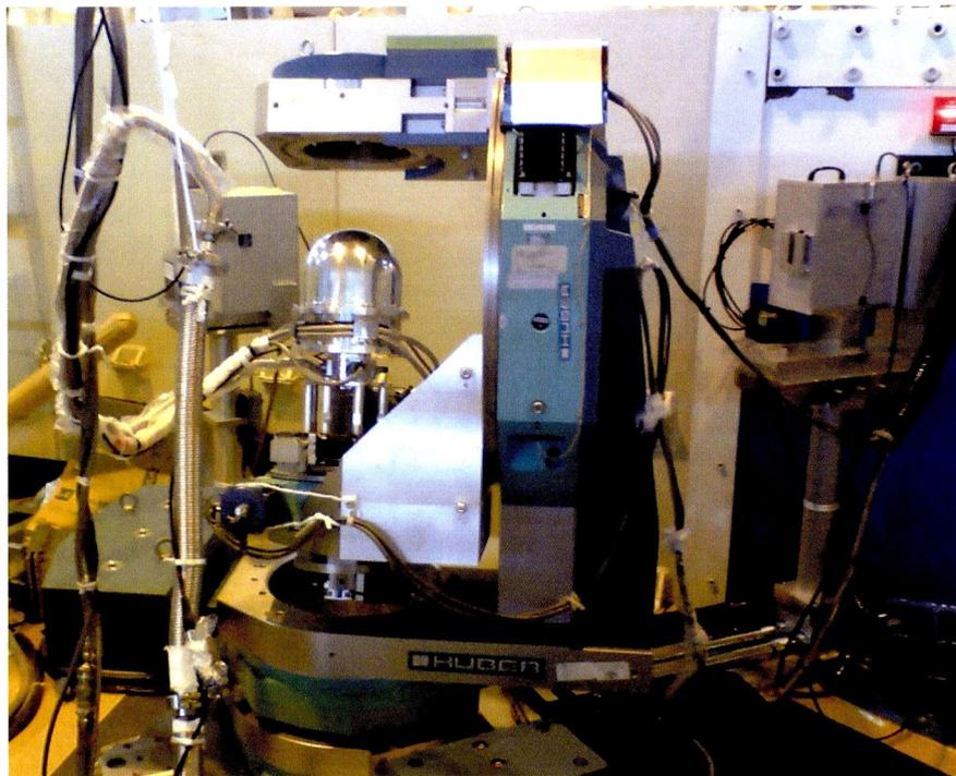
Figure 2.12 External view of FONDER. The aluminum cryostat is in sealed state. The neutron counter is in left top beyond the cryostat dome. A neutron beam hole is confirmed in right top of the picture. The neutron beam shutter is open, in which the red lamp is turning on.
