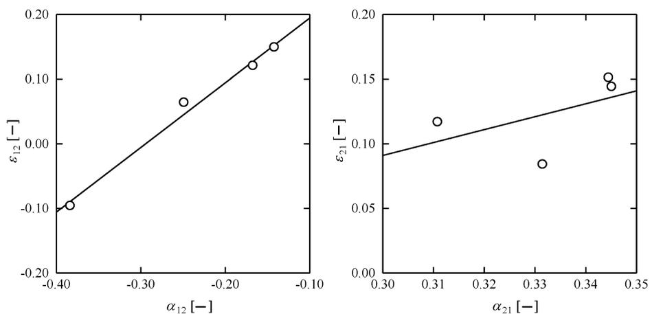
**Fig. 10** Relationships between  $\varepsilon_{12}$ ,  $\varepsilon_{21}$  and  $\alpha_{12}$ ,  $\alpha_{21}$  for water (1) + alcohol (2) systems;  $\alpha_{12} = 2.83 \times 10^{-3} t_{b,2} - 7.12 \times 10^{-4} \delta_{25,2}^2$  and  $\alpha_{21} = 1.84 \times 10^{-3} t_{b,2} + 2.84 \times 10^{-4} \delta_{25,2}^2$
