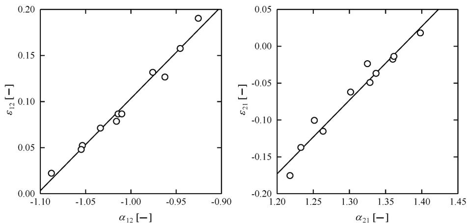
**Fig. 8** Relationships between  $\varepsilon_{12}$ ,  $\varepsilon_{21}$  and  $\alpha_{12}$ ,  $\alpha_{21}$  for ketone (1) + alcohol (2) systems;  $\alpha_{12} = -4.32 \times 10^{-3} t_{b,1} + 1.88 \times 10^{-3} t_{b,2} - 1.51 \times 10^{-3} \delta_{25,1}^2 - 4.66 \times 10^{-4} \delta_{25,2}^2$  and  $\alpha_{21} = 5.17 \times 10^{-3} t_{b,1} - 2.29 \times 10^{-3} t_{b,2} + 1.96 \times 10^{-3} \delta_{25,1}^2 + 6.50 \times 10^{-4} \delta_{25,2}^2$
