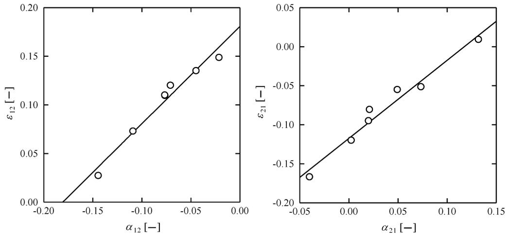
**Fig. 6** Relationships between  $\varepsilon_{12}$ ,  $\varepsilon_{21}$  and  $\alpha_{12}$ ,  $\alpha_{21}$  for cyclohexane (1) + paraffinic or aromatic hydrocarbon (2) systems;  $\alpha_{12}=1.08 \times 10^{-3} t_{b,2} - 6.53 \times 10^{-4} \delta_{25,2}^2$  and  $\alpha_{21} = -1.82 \times 10^{-3} t_{b,2} + 7.86 \times 10^{-4} \delta_{25,2}^2$
