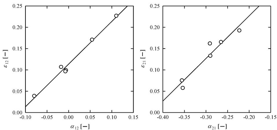
**Fig. 9** Relationships between  $\varepsilon_{12}$ ,  $\varepsilon_{21}$  and  $\alpha_{12}$ ,  $\alpha_{21}$  for ethanol (1) + hydrocarbon (2) systems;  $\alpha_{12} = 2.31 \times 10^{-3} t_{b,2} - 7.48 \times 10^{-4} \delta_{25,2}^2$  and  $\alpha_{21} = -2.20 \times 10^{-3} t_{b,2} - 3.21 \times 10^{-4} \delta_{25,2}^2$
