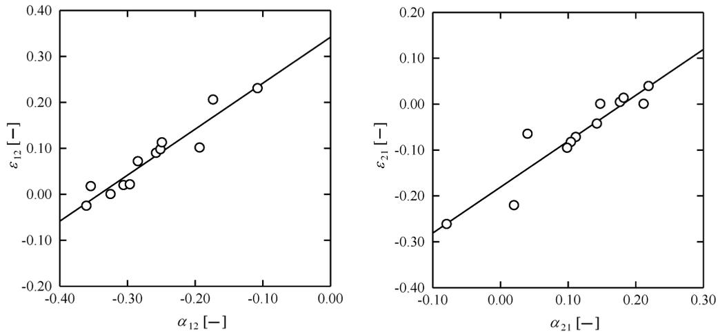
**Fig. 7** Relationships between  $\varepsilon_{12}$ ,  $\varepsilon_{21}$  and  $\alpha_{12}$ ,  $\alpha_{21}$  for ether (1) + paraffinic hydrocarbon (2) systems;  $\alpha_{12} = -2.64 \times 10^{-3} t_{b,1} + 2.18 \times 10^{-3} t_{b,2} - 1.46 \times 10^{-3} \delta_{25,1}^2 + 2.17 \times 10^{-4} \delta_{25,2}^2$  and  $\alpha_{21} = 2.73 \times 10^{-3} t_{b,1} - 2.42 \times 10^{-3} t_{b,2} + 1.58 \times 10^{-3} \delta_{25,1}^2 - 9.98 \times 10^{-4} \delta_{25,2}^2$
