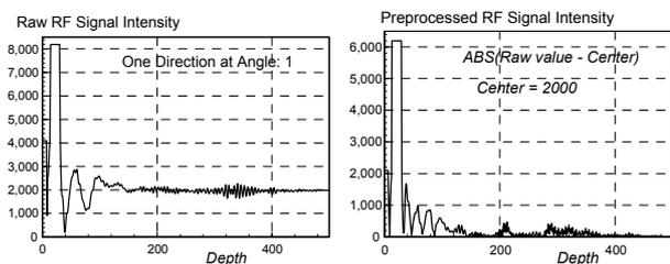
Fig. 1. The Raw and the Preprocessed RF Signal.
