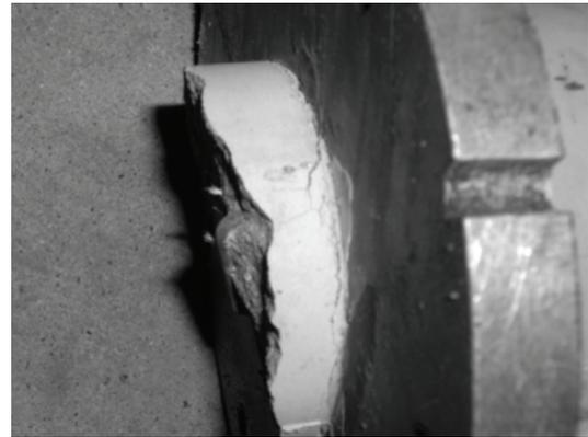
FIGURE 3: Typical failure within the end zone of the dog-bone-shaped specimen.
