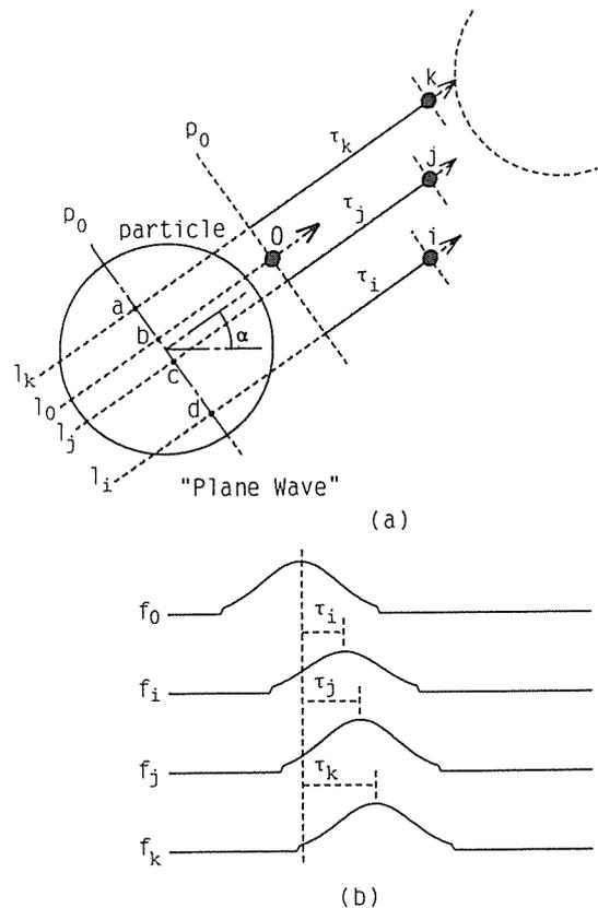
Fig. 3 Relation between lag time of the mutual-correlation function and particle motion. (a) If the particle has central symmetry of brightness distribution, passing of particle is equivalent to the passing of a "Plane Wave" (line  $p_0$  show a ridge of the wave). (b) Temporal brightness change at respective pixels.
