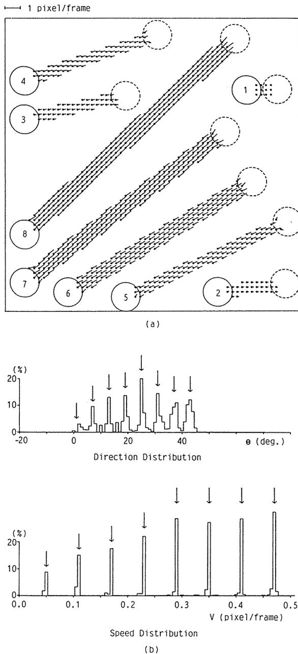
Fig. 5 Result of analysis of the artificial image. (a) Obtained optical flow. Given motion of particles are illustrated by solid circle (start position) and broken circle (end position). (b) Histograms of speed-distribution and angle-distribution of obtained optical flow. True data are indicated by arrows in the figure.
