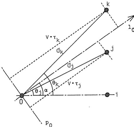
Fig. 4 Estimation of exact velocity at the target pixel. From the geometrical relations in the figure, we can estimate the moving velocity.
