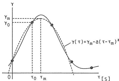
Fig. 2 Estimation of true lag time by a quadratic interpolation method.
