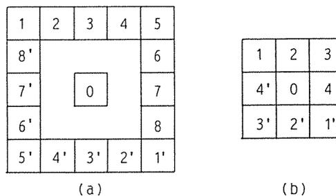
Fig. 1 A target pixel of velocity analysis and neighboring pixels. The local velocity at the target pixel (0) is evaluated by analyzing mutual-correlation functions between a temporal brightness change of the target pixel and that of the neighboring pixels. Motion of constant velocity is assumed in the localized area ( $5 \times 5$  or  $3 \times 3$  pixels-area is used for the analysis).
