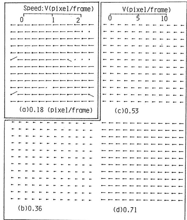
Fig. 4 Velocity-field representation of the simulation images with orientated lines. The length and the orientation of the lines represent the speed and the direction of particle movement, respectively. Given speeds are also shown in the figure.
