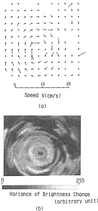
Fig. 6 Result of the velocity-field analysis of the vortex motion. (a)Representation of the velocity-field with orientated lines. Vacant pixel-sites show the position where the velocity can not evaluate because of no passing of particles. (b)“The variance image” of the vortex motion. Black regions in the image indicate no particle movement at the regions. The regions well coincide with the vacant pixel-sites in the upper figure (a).
