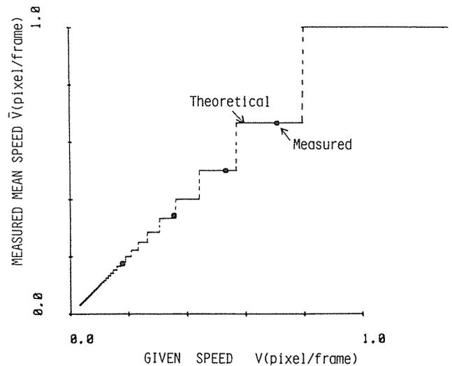
Fig. 5 Relation between the given speed and the measured mean speed. Stepwise line shows the theoretical value considering the digital error in the measurement.
