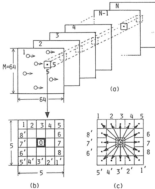
Fig. 1 Configuration of dynamic image. (a) A digital dynamic image with  $M \times M$  pixels and  $N$  frames. (b) A target pixel (0) and its next-nearest neighbouring 16 pixels. (c) A definition of 16 directions.
