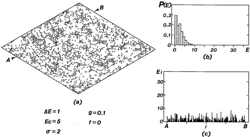
Fig. 4. Crack pattern and strain energy distribution for the system with  $\Delta E=1$ ,  $E_c=5$ ,  $\sigma=2$ ,  $g=0.1$  and  $f=0$ .
