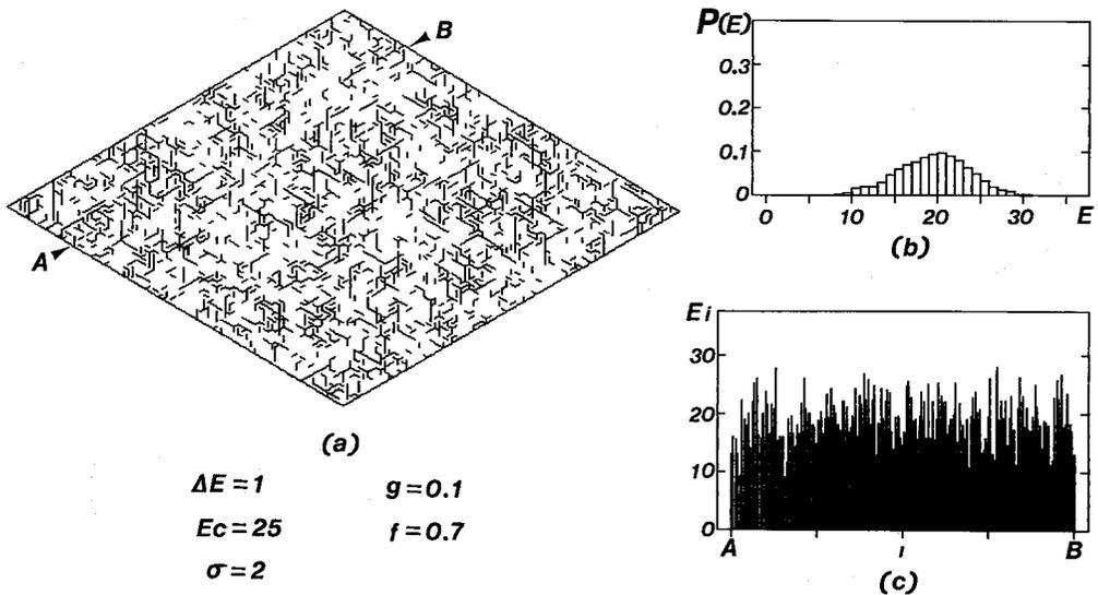
Fig. 6. Crack pattern and strain energy distribution for the system with  $\Delta E=1$ ,  $E_c=25$ ,  $\sigma=2$ ,  $g=0.1$  and  $f=0.7$ .
