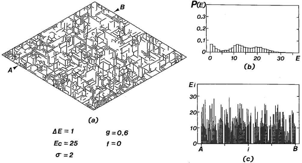
Fig. 5. Crack pattern and strain energy distribution for the system with  $\Delta E=1$ ,  $E_c=25$ ,  $\sigma=2$ ,  $g=0.6$  and  $f=0$ .
