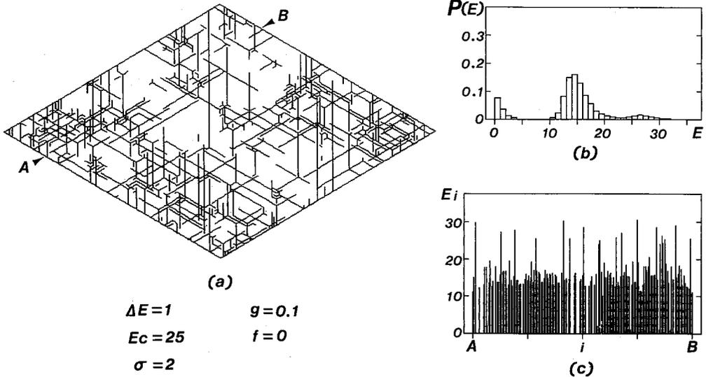
Fig. 3. Crack pattern and strain energy distribution for the system with  $\Delta E=1$ ,  $E_c=25$ ,  $\sigma=2$ ,  $g=0.1$  and  $f=0$ .
