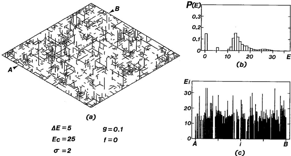
Fig. 7. Crack pattern and strain energy distribution for the system with  $\Delta E=5$ ,  $E_c=25$ ,  $\sigma=2$ ,  $g=0.1$  and  $f=0$ .
