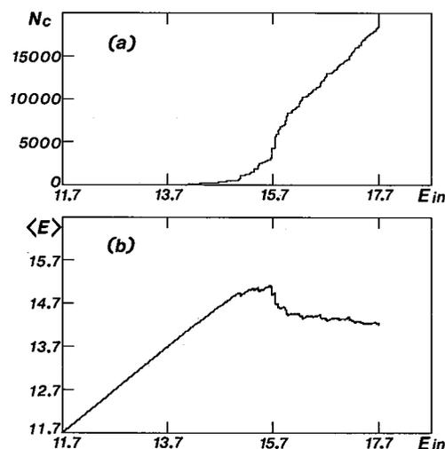
Fig. 2. Dependence of the number of cracks ( $N_c$ ) and the average strain energy per element ( $\langle E \rangle$ ) on the input strain energy ( $E_{in}$ ) per element for the system with  $\Delta E = 1$ ,  $E_c = 25$ ,  $\sigma = 2$ ,  $g = 0.1$  and  $f = 0$ .
