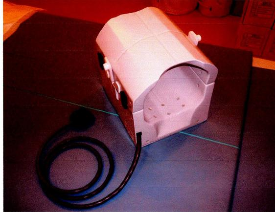
Fig.3: Quadrature detection (QD) coil for human stifle joint of AIRIS II comfort, Hitachi Medical Co., Tokyo, Japan.
