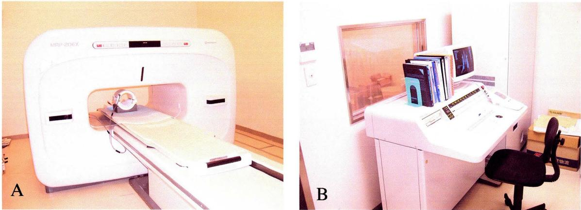
Fig.1: MRP-20EX, Hitachi Medical Co., Tokyo, Japan. 0.2 T permanent magnet system. A: Scan room. Widely opened gantry. B: Control room.
