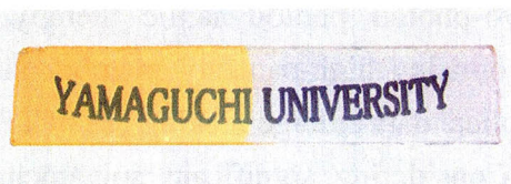
Figure 1. Photograph of the film deposited on a quartz substrate. The left side of the substrate was coated with a TPA compound solid film.
