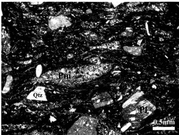
Fig. 7. Photomicrograph of welded tuff in the Futanoigawa Rhyolite Tuff Member. Qtz: quartz, Pl: plagioclase, Pm: pumice.
