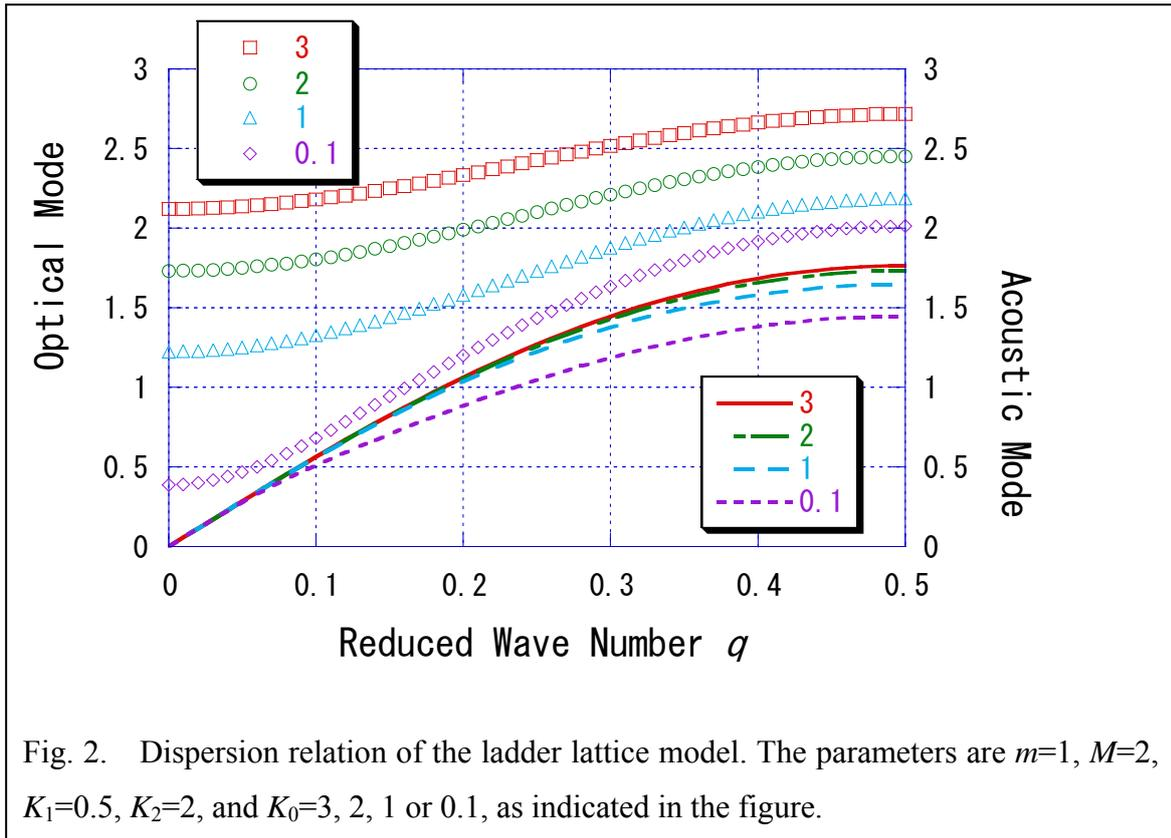
Fig. 2. Dispersion relation of the ladder lattice model. The parameters are  $m=1$ ,  $M=2$ ,  $K_1=0.5$ ,  $K_2=2$ , and  $K_0=3, 2, 1$  or  $0.1$ , as indicated in the figure.
