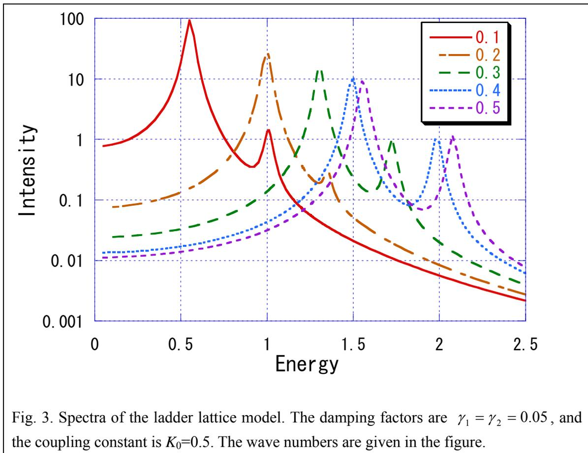
Fig. 3. Spectra of the ladder lattice model. The damping factors are  $\gamma_1 = \gamma_2 = 0.05$ , and the coupling constant is  $K_0=0.5$ . The wave numbers are given in the figure.
