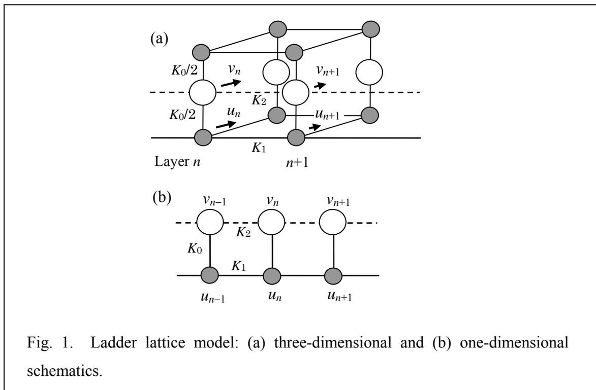
Fig. 1. Ladder lattice model: (a) three-dimensional and (b) one-dimensional schematics.
