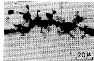
Fig. 16 Micro crack initiated at inclusions ( \text{MnAl}_6 ) during tensile test on a specimen heated 60 days at 100°C.
