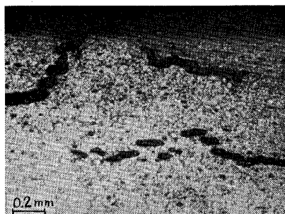
Fig. 12. The blisters in H.T. 80, as received by cathodic hydrogen charging. (3000 min)
