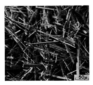
Fig. 1. Scanning electron micrograph of acicular crystals of compound Cu<sub>8</sub>Bi<sub>8</sub>S<sub>19</sub> synthesized at 460°C.
