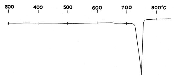
Fig. 4. Differential thermal curve for synthetic FeBi<sub>4</sub>S<sub>7</sub>
