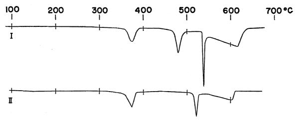
Fig. 3. The curves of differential thermal analysis for synthetic CuBiS<sub>2</sub> (emplectite)
