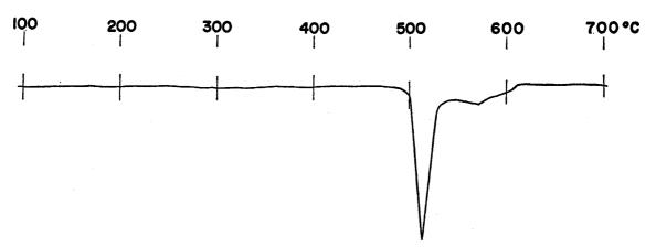
Fig. 2. Differential thermal curve for synthetic Cu<sub>8</sub>Bi<sub>8</sub>S<sub>19</sub>.
