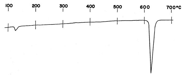
Fig. 6. The curve of differential thermal analysis for synthetic Cu<sub>3</sub>SbS<sub>3</sub>.
