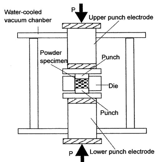
Fig.1 Schematic illustration of SPS apparatus.
