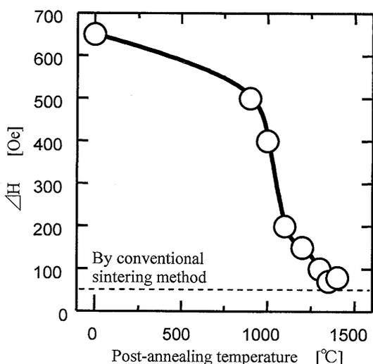
Fig.5 Annealing temperature dependence of  $\Delta H$ .
