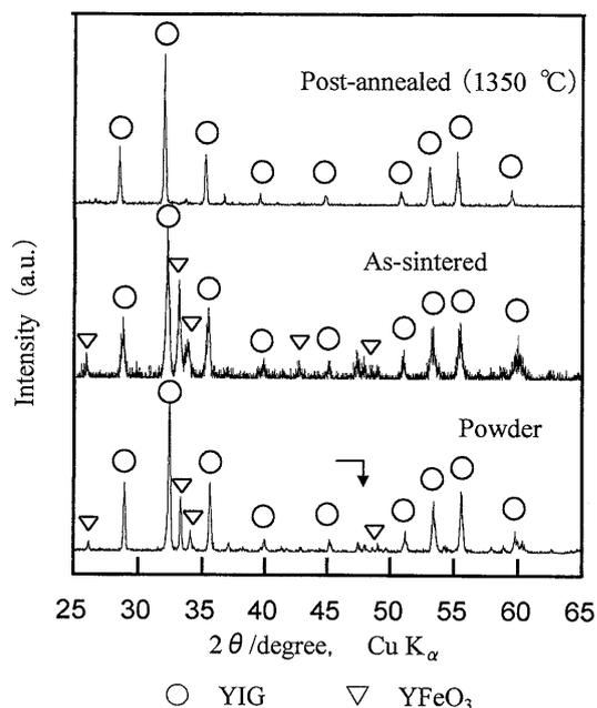
Fig.6 XRD diagrams for post annealed sample (top), as-sintered (middle), and powder of starting method (bottom).
