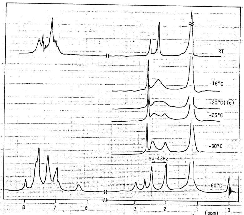
Fig. 2 Temperature dependence of 1 H NMR spectra of [5] in CDCl 3 .
