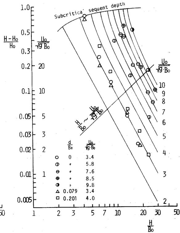
Fig. 22 Correlation of  $(H - H_0)/H_0$  and  $H/B_0$ .
