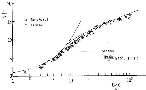
Fig. 15 Velocity profile of boundary layer along the Smooth wall.
