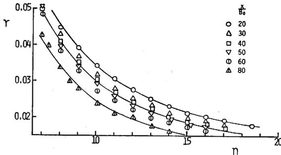
Fig. 11 Correlation of  $n$  and  $\gamma$  ( $n$  is exponents of power laws and  $\gamma$  is coefficients of friction laws)
