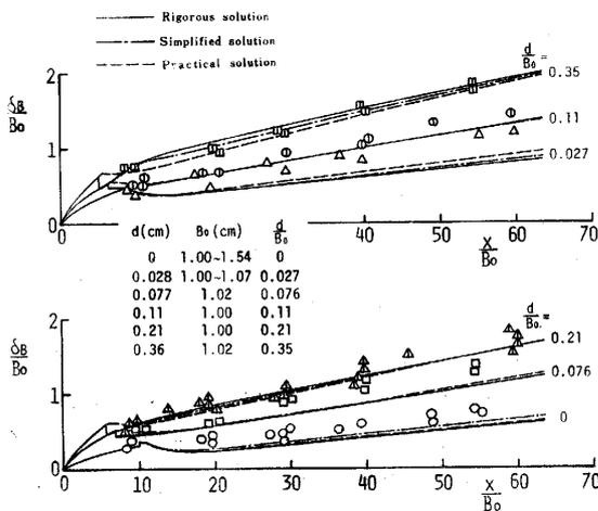
Fig. 17 Boundary layer growth in plane wall jets.
