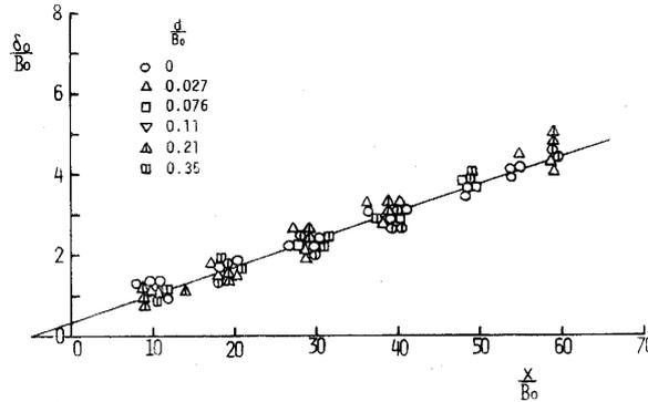
Fig. 8 Growth of the length scale in plane wall jets.
