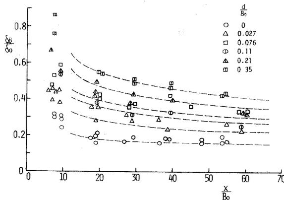
Fig. 7 Relative variation of characteristic length between the main flow and the boundary layer flow.
