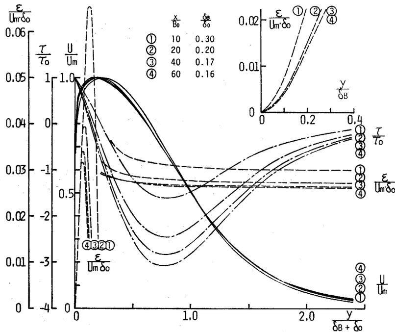
Fig. 13 Distributions of shear stress and eddy viscosity coefficient in plane wall jets along the smooth wall.
