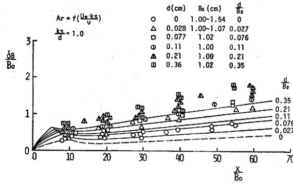
Fig. 10 Boundary layer growth in plane wall jets.
