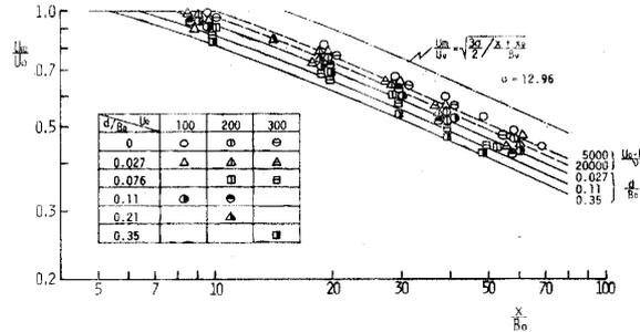
Fig. 9 Decay of maximum velocity in plane wall jets.
