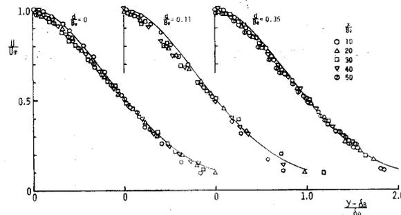
Fig. 5 velocity profiles in a main flow of the wall jet.
