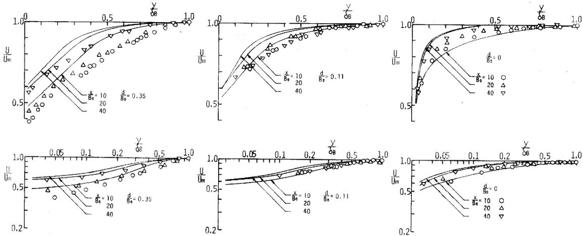
Fig. 19 Velocity profiles in plane wall jets.
