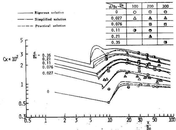
Fig. 18 Friction coefficient in plane wall jets.
