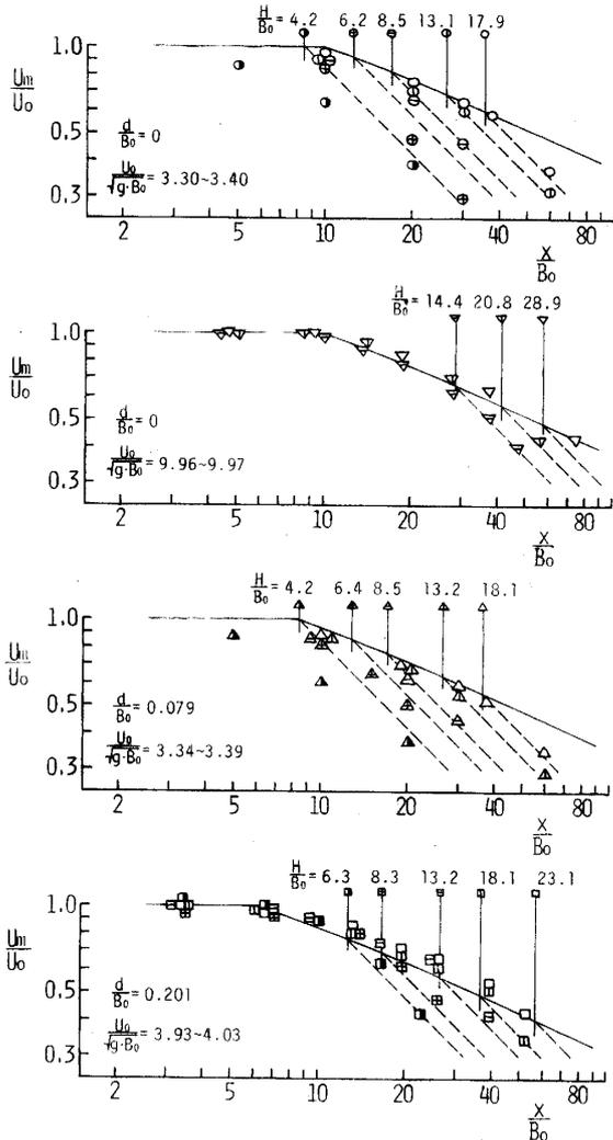
Fig. 23 Decay of the maximum velocity in the case of considering influences of downstream current depth.
