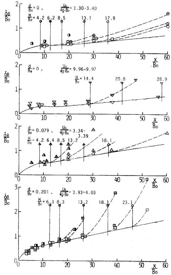
Fig. 24 Boundary layer growth in the case of considering influences of downstream current depth.
