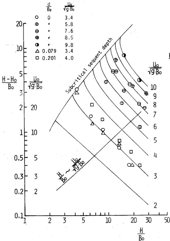
Fig. 21 Correlation of  $(H - H_0)/B_0$  and  $H/B_0$ .
