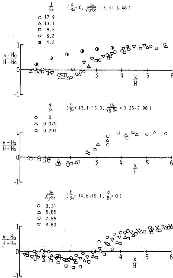
Fig. 20 The state of water surface downstream of a sluice.
