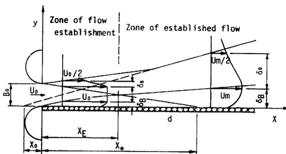
Fig. 3 Definition sketch of plane turbulent wall jet.
