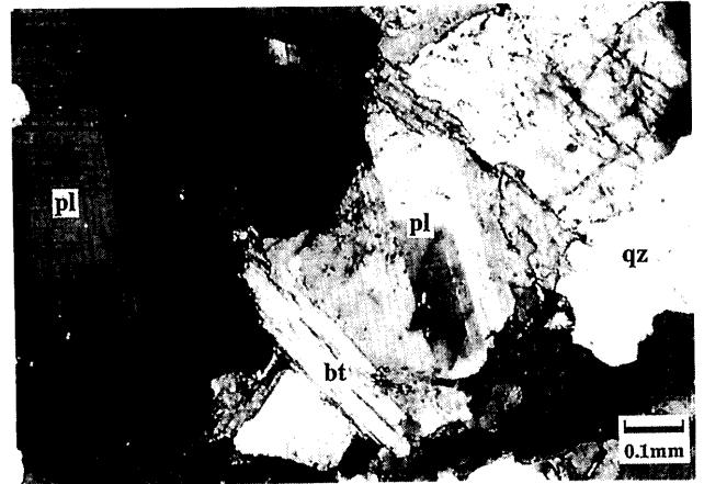
Photo.5 Photograph of polarization microscope of biotite granite sampled at Kumage (cross nicol);qz,quartz;pl,plagioclase ;bt,biotite
