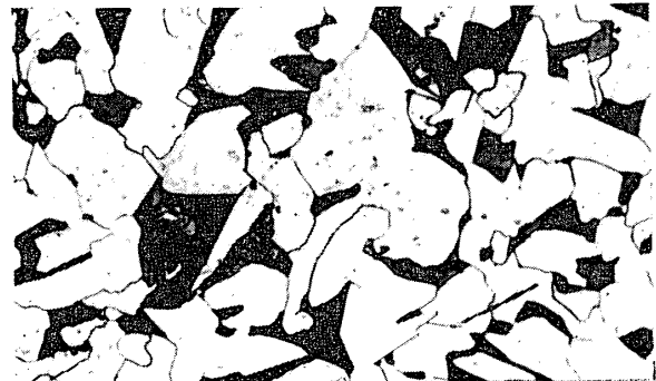
Fig. 2 (a) Microstructure of SM41A (as received). ( \times 200 )
