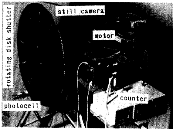
Photo. 2 Apparatus for measuring the velocity of waterdrop
