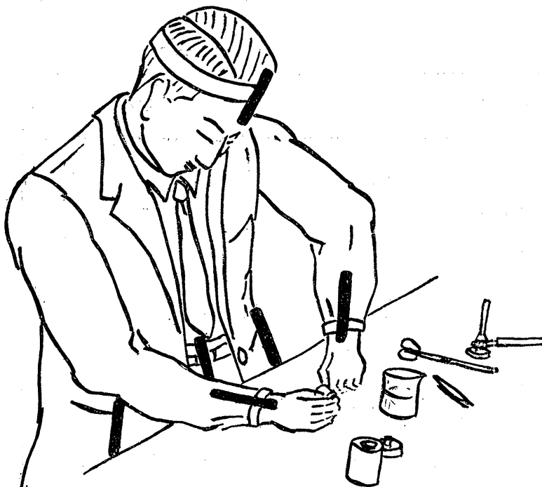
Fig. 6 Referential schema for Table IX. Shows a form which is handling the radium shells with pocket chambers on his body for measuring the radiation quantities from the radium
