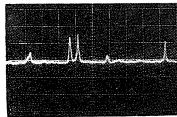
Fig. 8 Probe current wave form of conductivity measurement. N-5, gas flow rate 20 l/min arc current 100 A sweep velocity; 200 \mu\text{s}/\text{CM} gain; 5 V/CM
