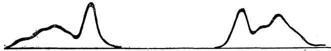
Figure 7. Electrophoretic pattern of fraction Al_3 -AcT. (Slightly modified). Explanation, see text. Veronal buffer. 14 mA., 180 V. 45 min.
