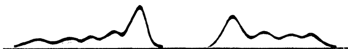
Figure 5. Electrophoretic pattern of fraction Al_3 . (Slightly modified) Explanation, see text. Veronal buffer. 14 mA., 180 V. 60 min.
