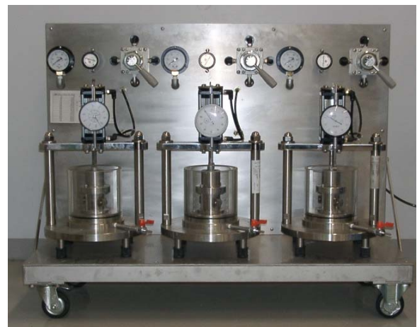
Photograph 2 Consolidation apparatus for cement stabilized soil
