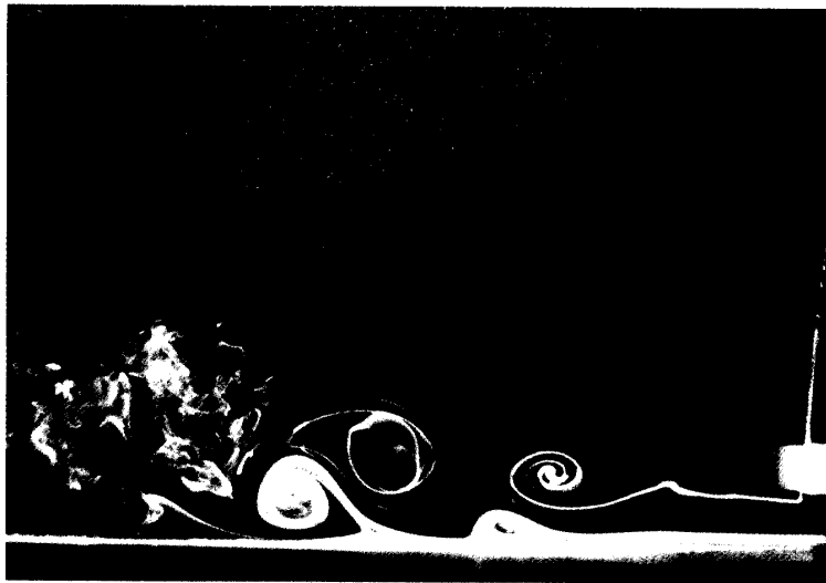
Fig. 9 Flow visualization of a pair vortex
