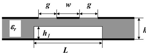
Fig. 2 Geometry of grooving CBCPW.
