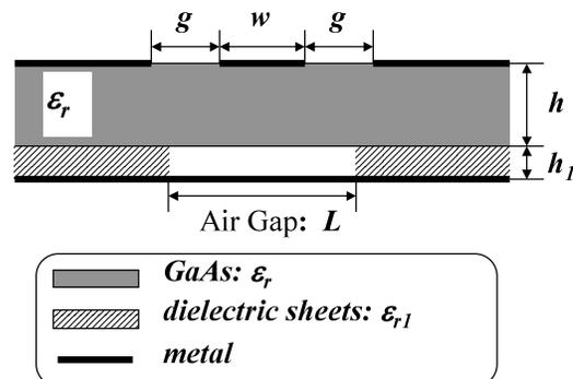
Fig. 4 Geometry of proposed AGS dielectric sheets backing CBCPW.
