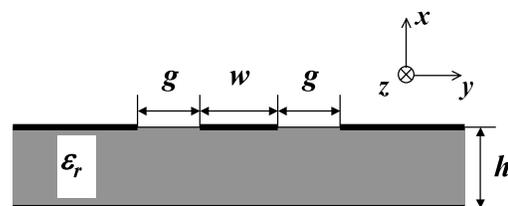
Fig. 1 Geometry of conventional CBCPW.
