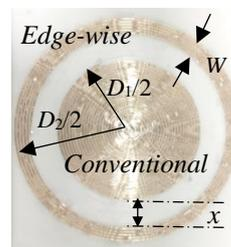
Fig.2 Dual-Spiral Resonator
