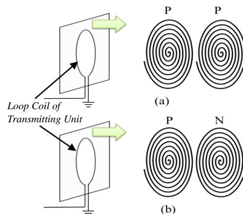
**Fig.3** Example setup for paired-spiral resonators with PP or PN winding direction
