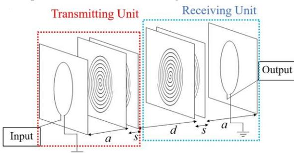
**Fig.1** Structure of RC-WPT system using paired-spiral resonators.
