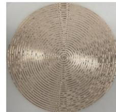
**Fig.2** Spiral Resonator
