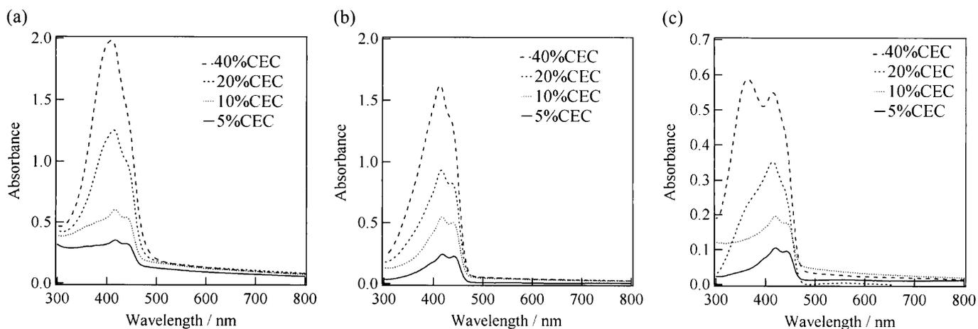
FIG. 3. Absorption spectra of Mont (a), SSA (b), SST (c) hybrid film fabricated at 5, 10, 20, 40%CEC.
