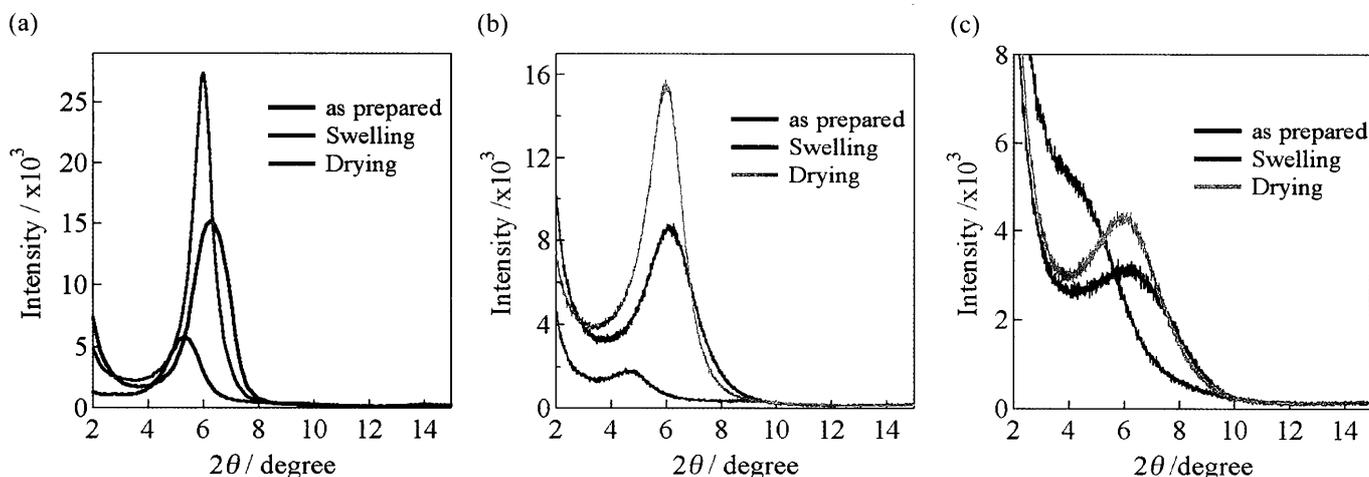
FIG. 4. XRD pattern of Mont (a), SSA (b), SST (c) hybrid film fabricated at 10%CEC of as prepared, swelling and drying state.
