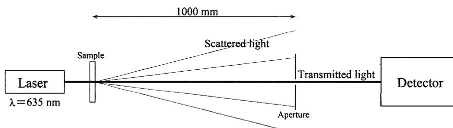
FIG. 2. Schematic representation of optical setup for measurement of transmittance.
