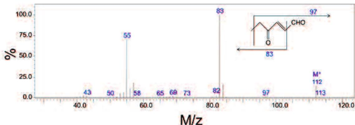
Figure 2-9. Mass spectrum of the compound at retention time of 17.59 min. assigned as 4-oxo-(*E*)-2-hexenal.
