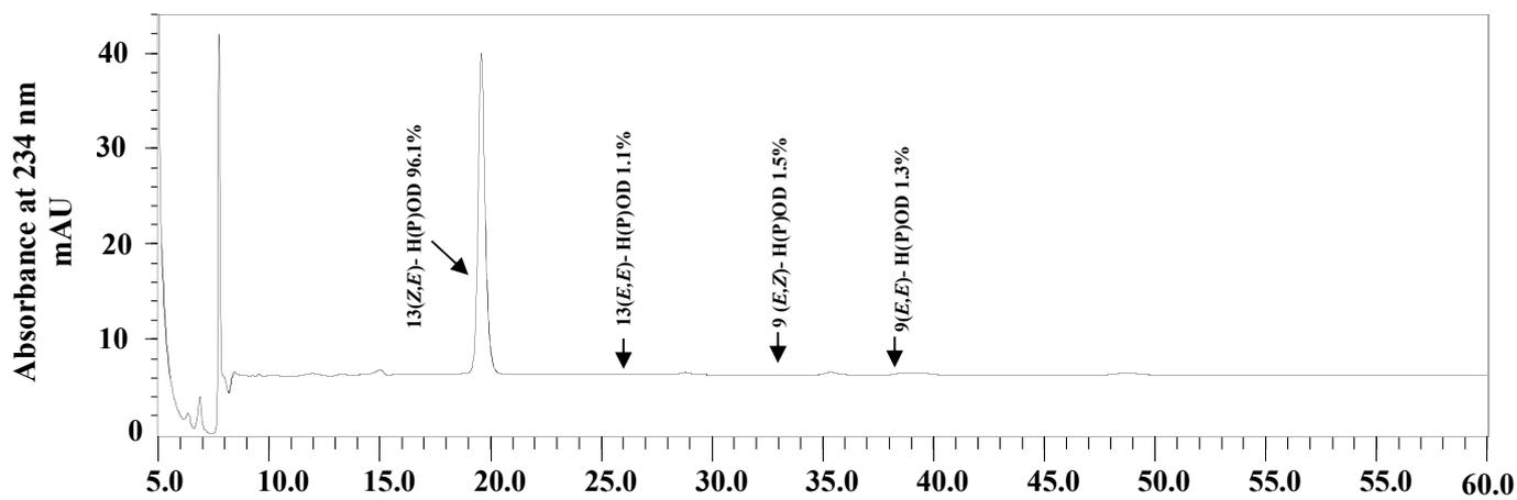
Figure 1-10. HPLC result showing the product of linoleic acid (18-2) with MpLOX7.
