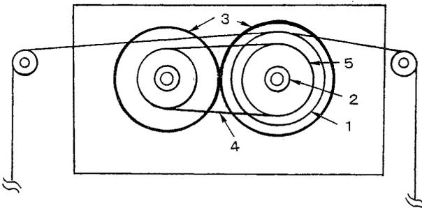
Fig.5 Improved energy converter element. 1: pulley to intake wave power, 2:one-way clutches, 3:gears, 4:chain, 5:sprocket
