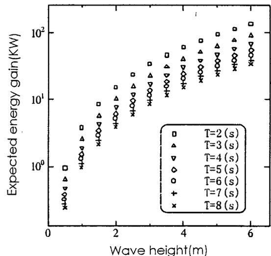
Fig.7 Expected energy gain. Float diameter 4m.
