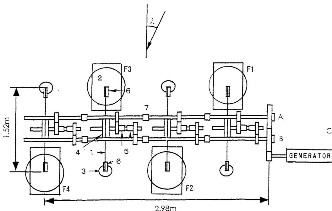
Fig.1 Simplified plans view of an experimental model. 1:wire, 2:float, 3:counter-weight, 4:pulley to extract wave power, 5:one-way clutches, 6:free pulley, 7:chain coupling, F1~F4 : floats.
