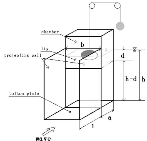
Fig.2 Schematic view of model caisson
